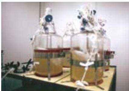
**Photo 2:** Insect cells (Sf-9) cultured in 20-L polypropylene bioreactors, with a 7-L culture volume
