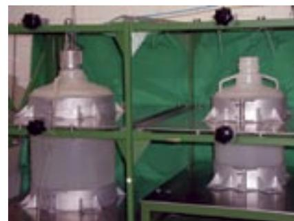
Photo 1: 50-L (left) and 20-L bioreactors mounted on a standard RC-6 shaking machine (Kühner AG, Switzerland). The shaking machine has a fixed shaking diameter of 50 mm.
