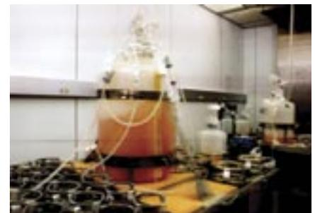
**Photo 4:** Hybridoma cells cultured in a 50-L polypropylene bioreactor, with a 36-L culture volume (see reference 7 for details)
