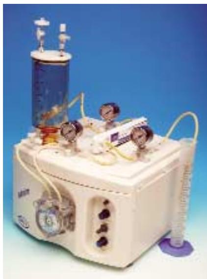
**A Minimate TFF Capsule device for development and processing applications using small sample volumes. Samples can be concentrated down to about 5 mL and diafiltered.**
