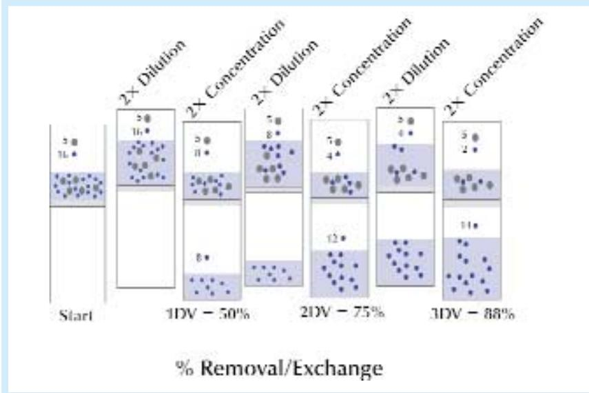
**Figure 3:** Discontinuous diafiltration (sequential dilution). Large circles represent molecules that are bigger than the pores in the membrane, and small circles represent molecules (such as salts or solvent) that are smaller than those pores.
