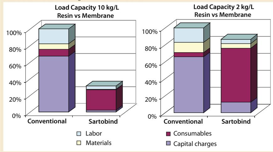
membrane chromatography is used in place of resin-based chromatography. Overall operating costs for the FT AEX step are reduced in spite of increased consumable costs, although there is an economy of scale that was not considered in the evaluation. Media costs increase because a new membrane chromatography capsule is used for each chromatography cycle. Conversely, a column is reusable and can be cycled up to 100 times.
