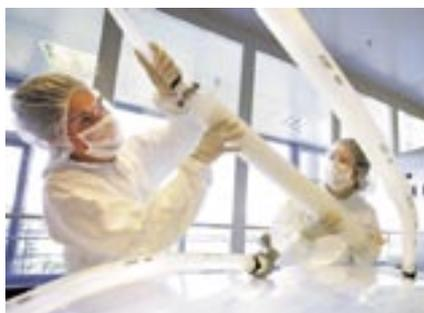
**Photo 1:** Purification associates are handling a 30-in Q membrane chromatography device. It can be used for virus clearance and trace contaminant removal at large scale.
