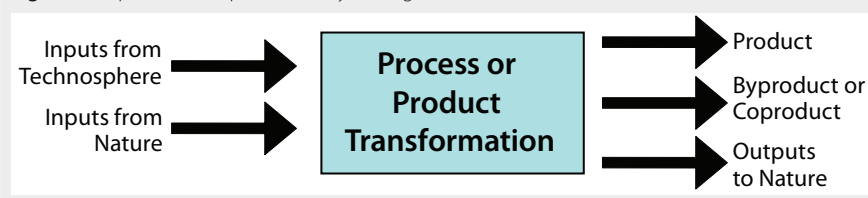
Figure 1: Inputs and outputs of life-cycle stages
